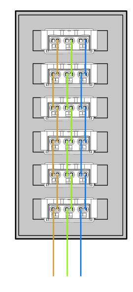
Wiring: H07V-U 2.5mm2 Free wire end length: 100mm
