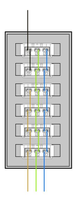
Wiring: H07V-U 2.5mm2 Free wire end length: 100mm
