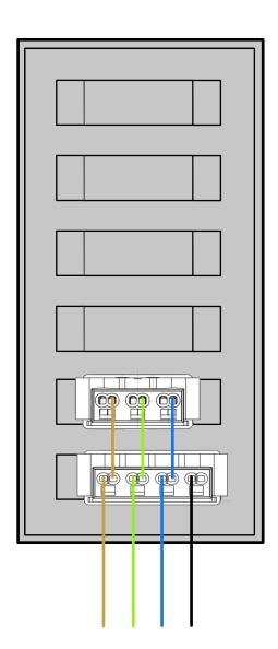
Wiring: H07V-U 2.5mm2 Free wire end length: 100mm
