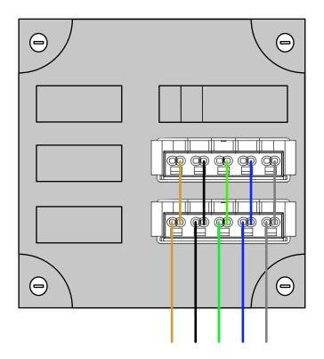
Wiring: H07V-U 2.5mm2 Free wire end length: 100mm
